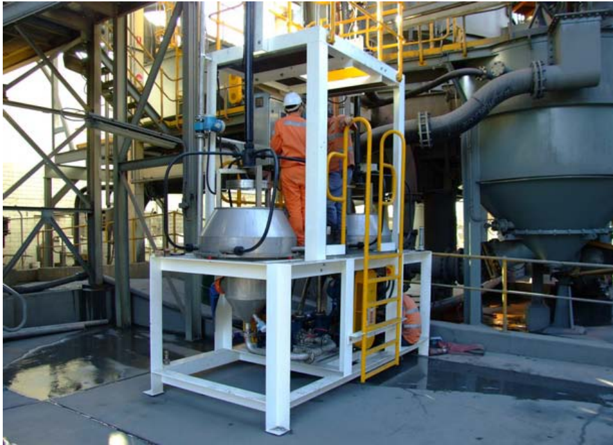
Figure 15.0 Imhoflot G10 Two Cell Pilot Plant in Operation
