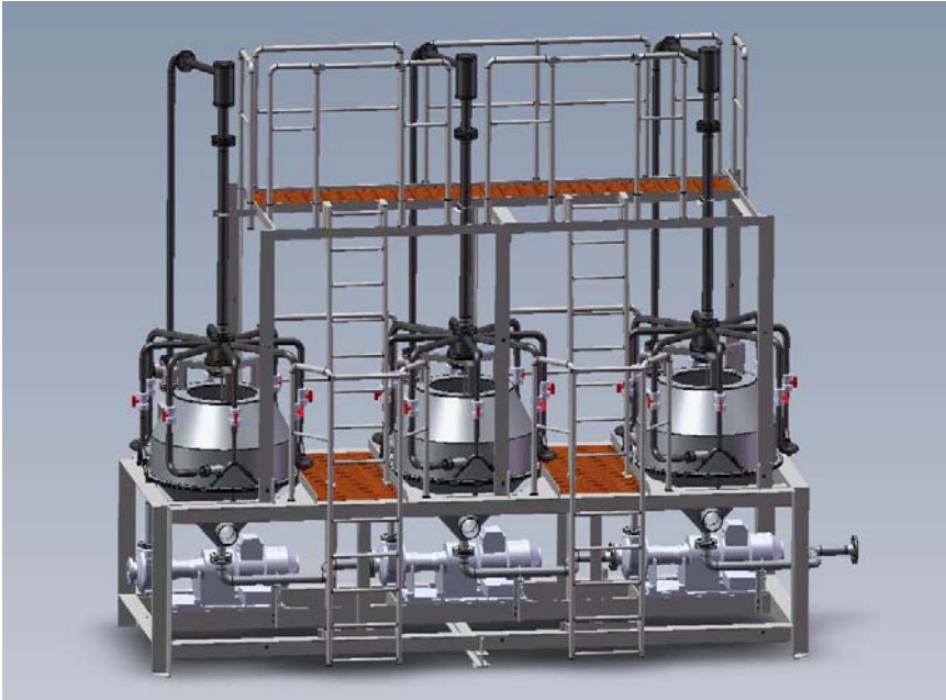
Fig 8.0 Schematic of Imhoflot 3 Stage G 12 Pilot Plant
