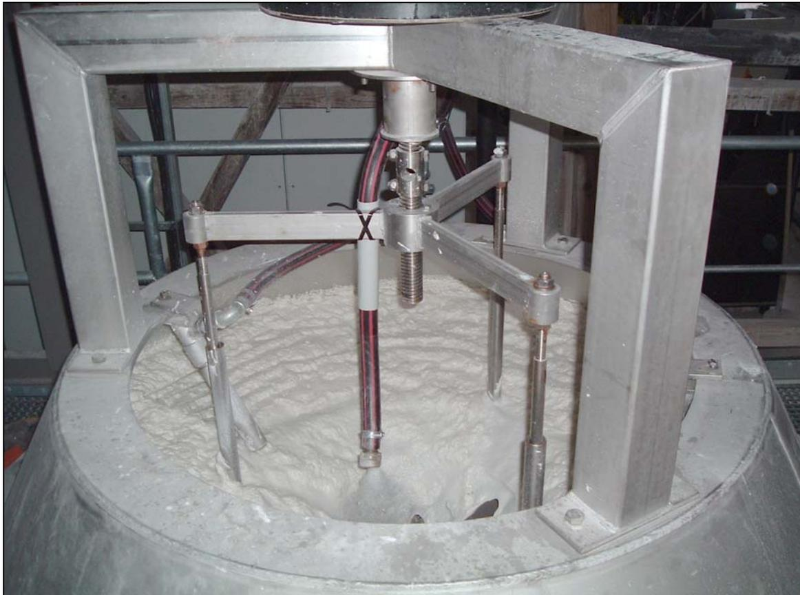
**Figure 9: Kaolin flotation at Dorfner**
