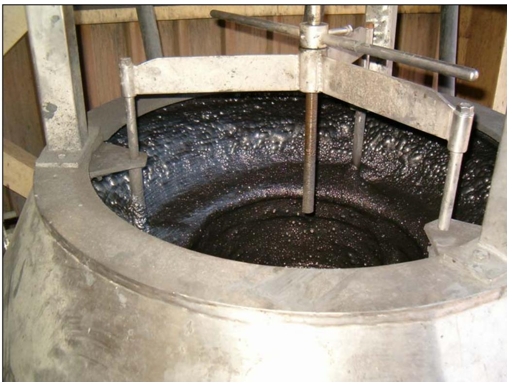
**Figure 3: Flotation froth produced at the Barbrook Gold Mine**
