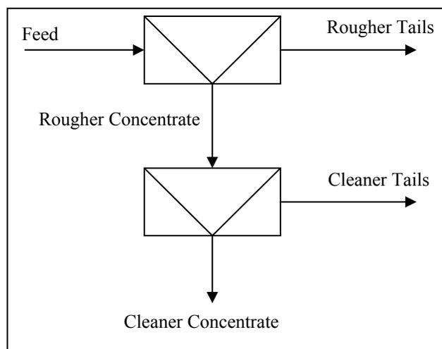
**Figure 4 : Laboratory flotation procedure followed**
