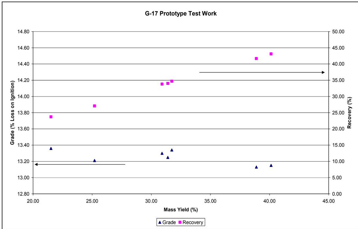
**Figure 5: Results obtained from pilot plant test work**
