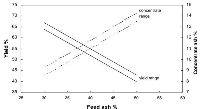
Figure 6. Flotation Recovery and Grade Relationships
