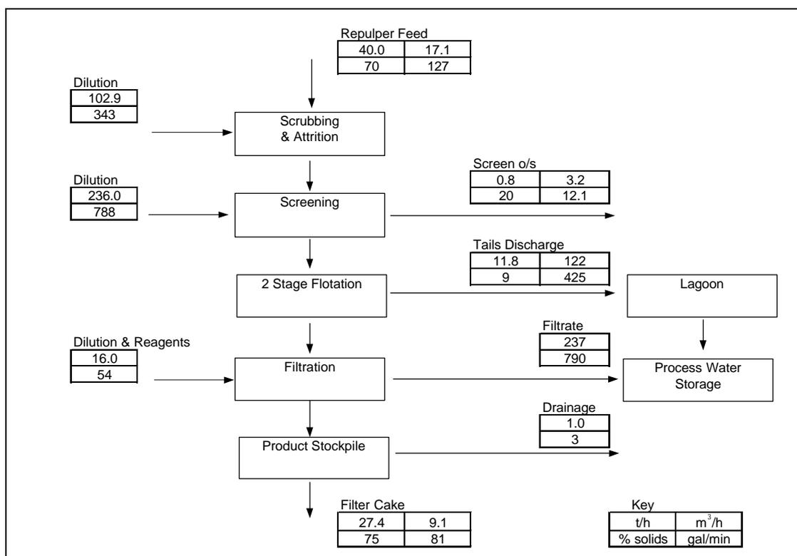
Figure 7. Process Flow Diagram and Typical Mass Balance
