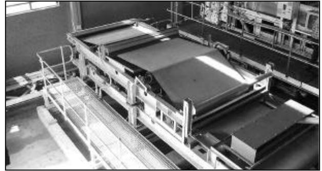
Figure 5. PSS Steel Belt Filter Model SBF1900
