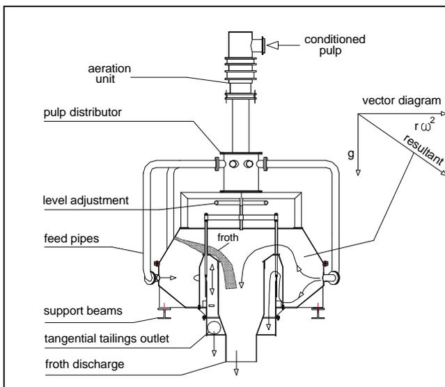
Figure 1. Imhoflot G Cell Schematic Diagram
