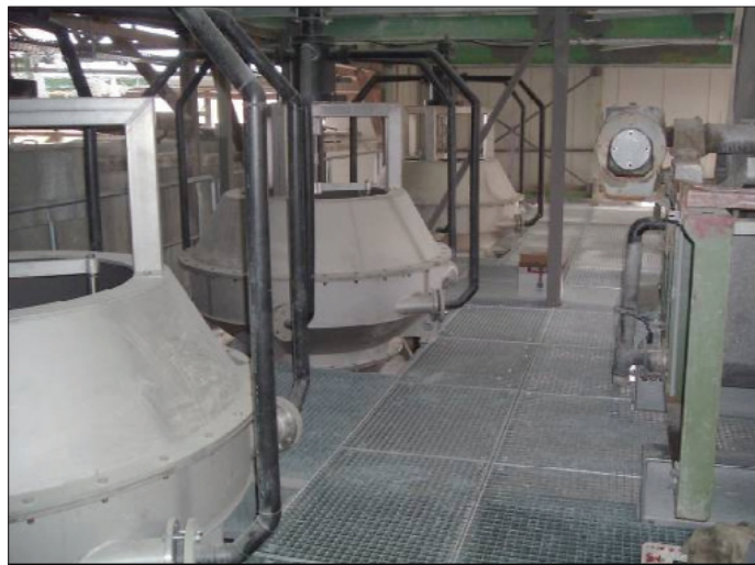
Figure 4—Dornier flotation plant showing the 3 G-Cells in series
