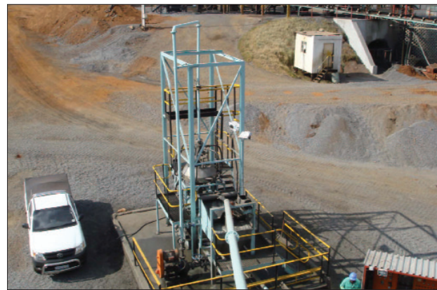
Figure 9—G-Cell and feed box arrangement
