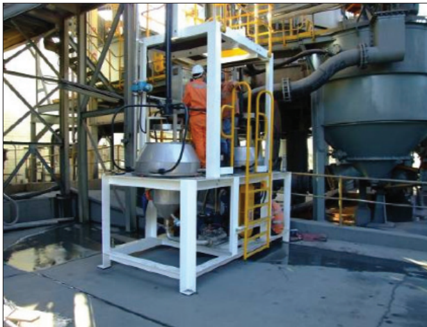
Figure 13—G-10 Pilot plant on the mobile rig for easy transport and operation
