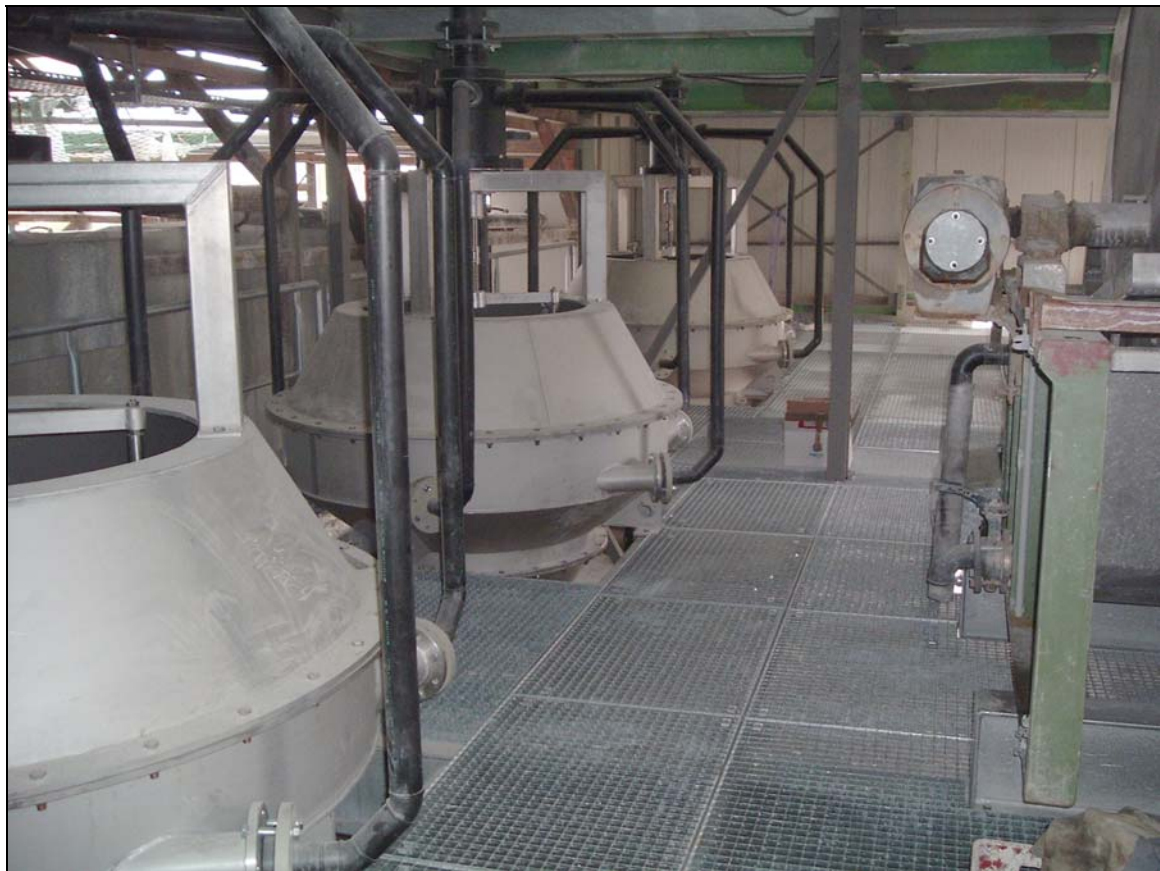
Figure 7: Dorfner flotation plant showing the 3 G-Cells in series
