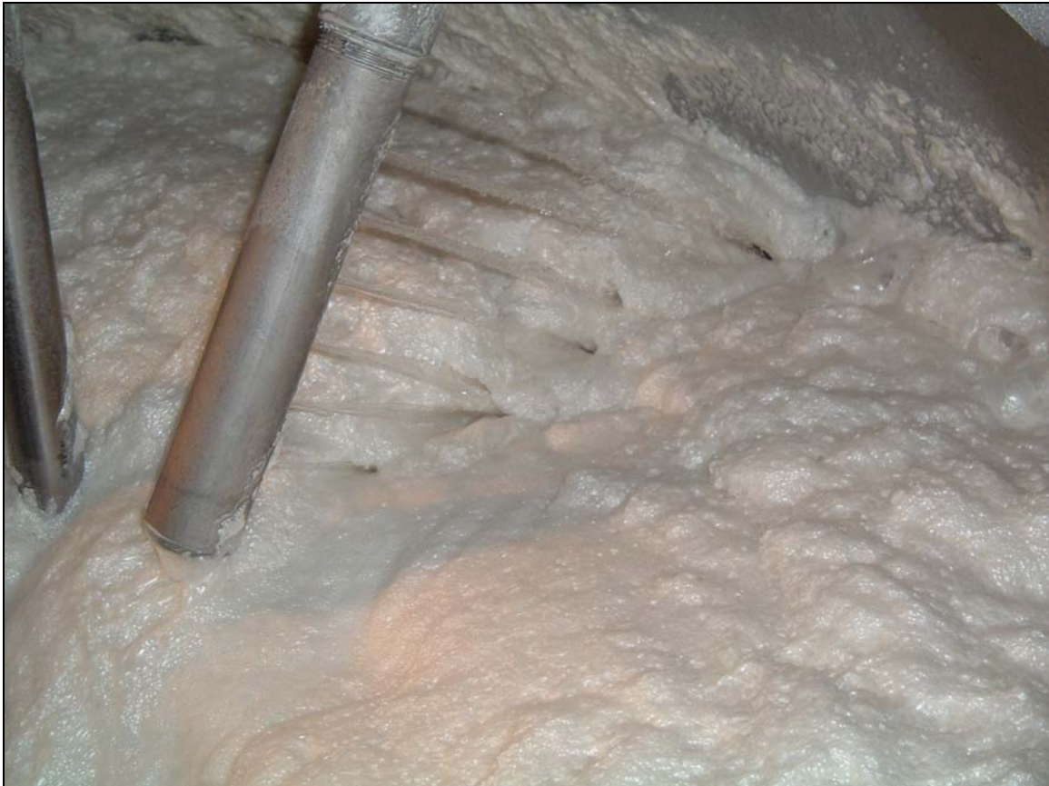
Figure 10: Froth washing of the concentrate to produce the required grade
